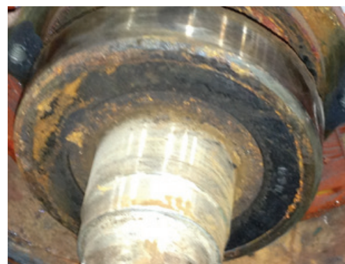
Figure 2: Damaged bearing in the electric motor from ingress of cooling solution
