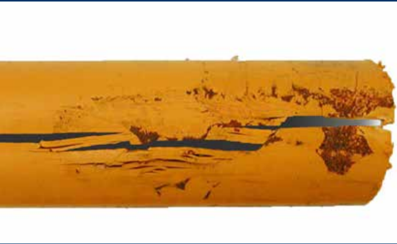
The above pipe was installed in contact with plasticizers
